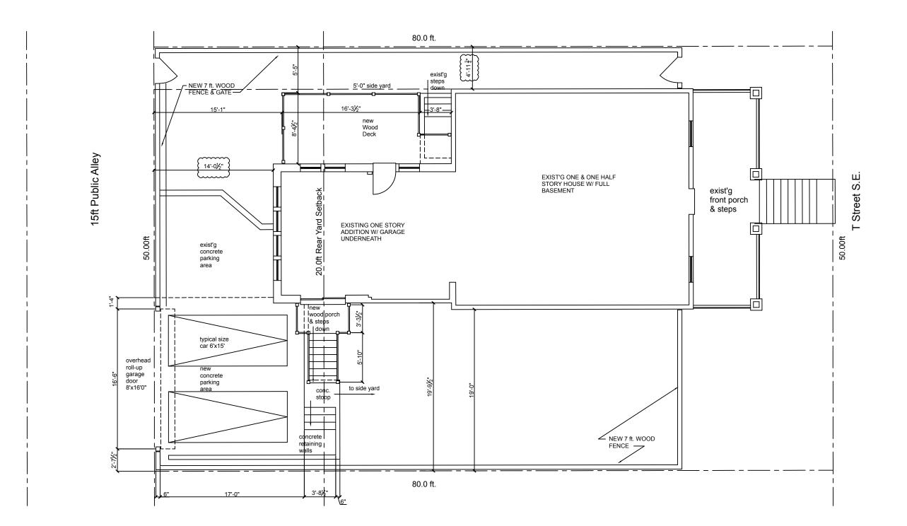
Site Plan - existing House with new side Porch & Deck scale: 1/8" = 1'-0"
